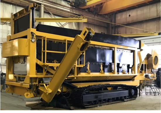
Roll off refractory lined "Air Curtain Burner" making biochar from forest residues, Oregon
